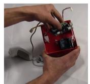
**Step 8:** Remove Arduino board from metal box. Note that it will take some force to remove it.
