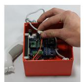
**Step 4:** Detach controller cable from remote connector.
