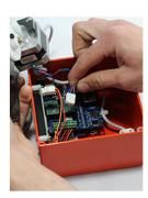
**Step 3:** Detach LCD cable from TB3 Orange board to LCD.
