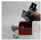
**Step 2:** Detach motor cable from TB3 Orange board. Remove entire top plate.
