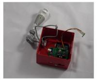
**Step 11:** Once Upgrade Kit is secured to metal box, bend 3-lead voltage regulator into upright position pressed against metal wall.
