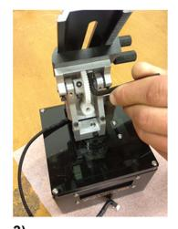
Tighten screw connecting the Fotomate to the TB3. Hand tighten. This doesn't need to be over tightened as you may want to replace this camera plate in the future.
