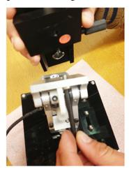
Insert the screw and align the Fotomate with the TB3 tilt head.
