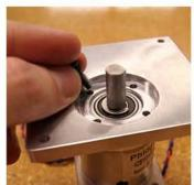
**Step 2:** Mount the adapter plate and the geared stepper motor to the Stage 0 carriage using the thumb screws in the orientation seen to the right.
