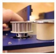
**NOTE:** When removing and installing pulleys, on any motor, there is a risk of marring the shafts, which can later make pulley removal difficult. When removing the pulley, always make sure both set-screws are fully disengage.
