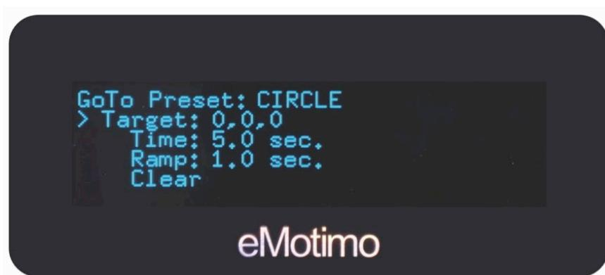
**1.Target:** Set your target parameter by moving all 4-axis to a position you want to lock in as a preset. Press X to lock in this position.
