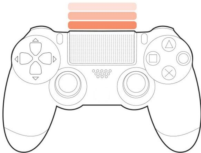
**ERROR: Fast Red Flash:** Error conditions over-voltage or under-voltage. Check power source.
