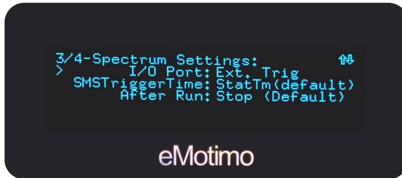
**I/O Port:** The i/o port allows spectrum ST4 to take in communication from 3rd party devices. The options are:
