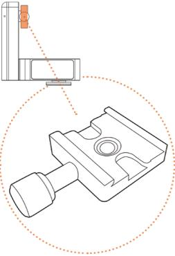
Arca plate mounted to spectrum pan base
