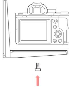
**Step #3** Mount camera and L-plate to tilt clamp.
