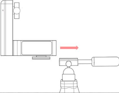
**Step #2** Mount camera to arca compatible L-plate.
