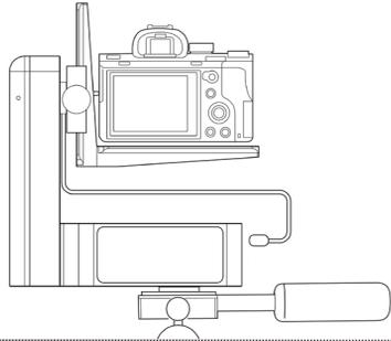
**Step #5** Plug in 12-24 volt power and immediately press and release the center PS button. Remote shows blue LED when connected.
