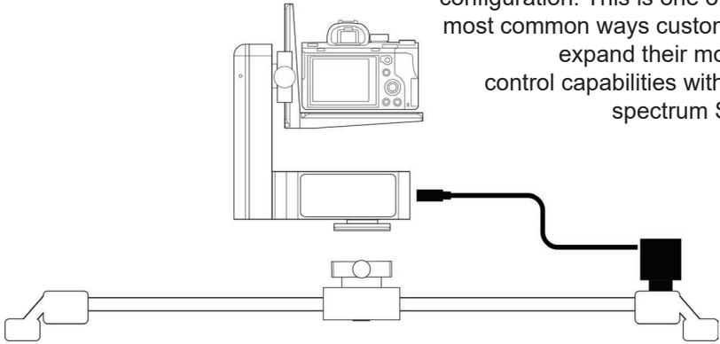
The **eMotimo focus FZ** accessory will plug into the M3 or M4 port on the spectrum to enable live control of focus, or use key frames, stops, and presets to hit your marks every time.
