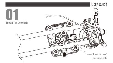
First install the belt to the fixator and lock to fix one side of the belt. Loop the drive belt around the first drive wheel.
