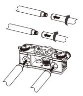
To install the extension tube, simply screw the additional rails on clockwise. Additional rail tubes can be purchased separately
